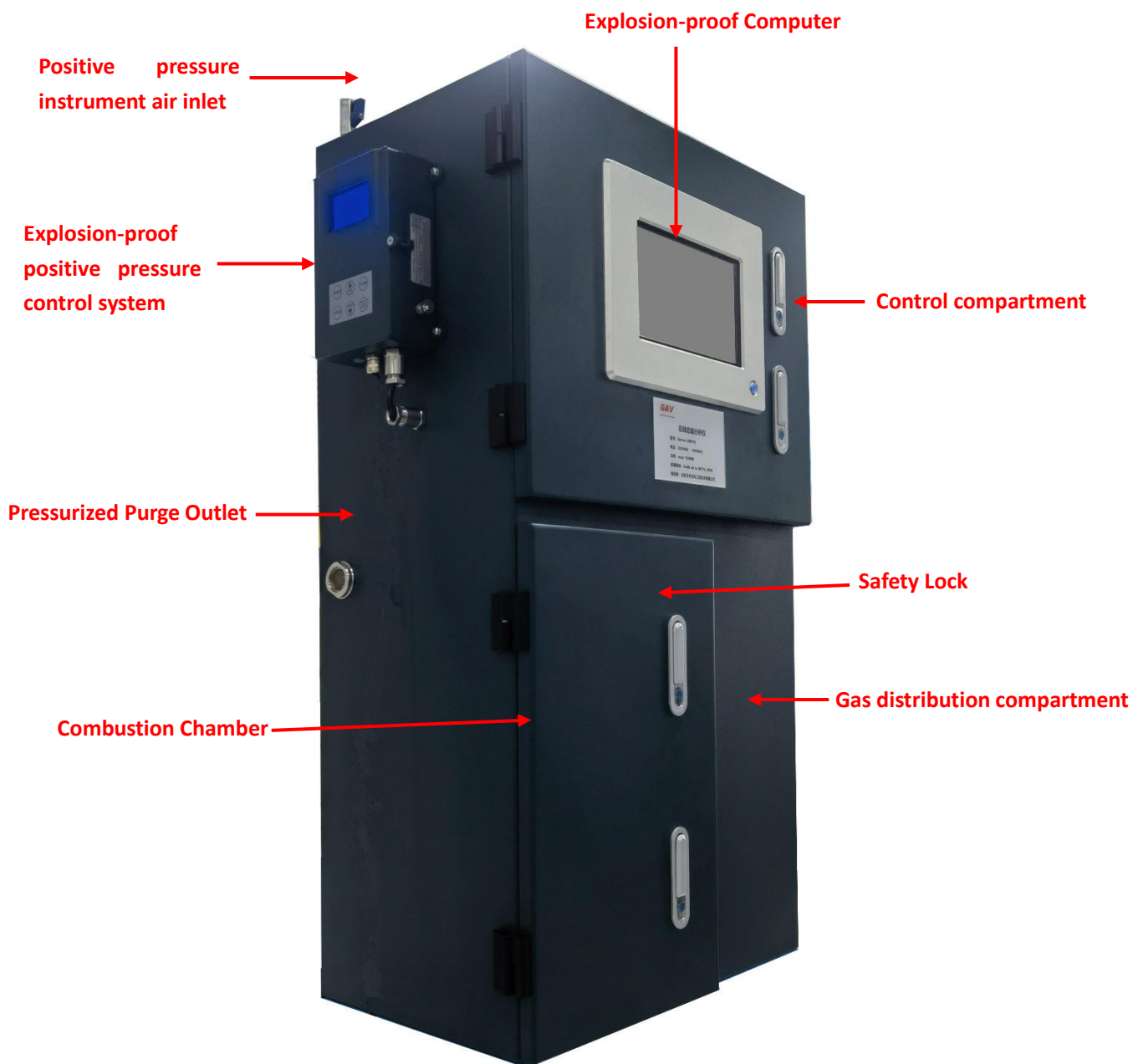
Series 800TS Sulfur On-Line Analyzer - Front View
